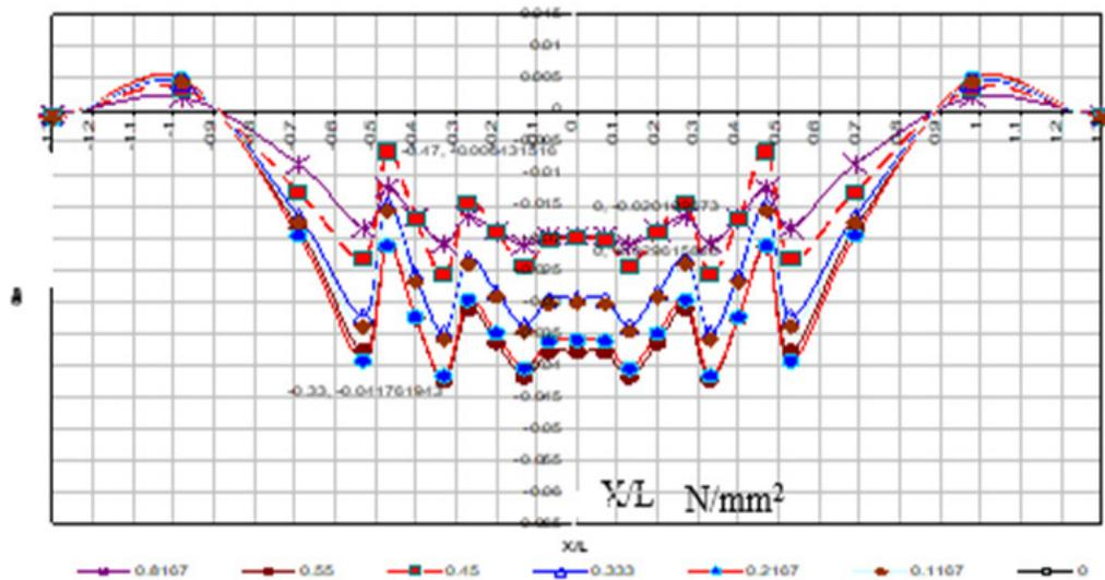
Fig. 11. Vertical stresses in  $N/mm^2$  linear SSI analysis (a) Contours of vertical stresses at footing level (b) Vertical stresses along longitudinal section at centre (c) Vertical stresses at foundation level along longitudinal sections for different values of  $Z/L$ .
