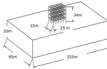
Fig.1. Structure-footing-soil system [5].
