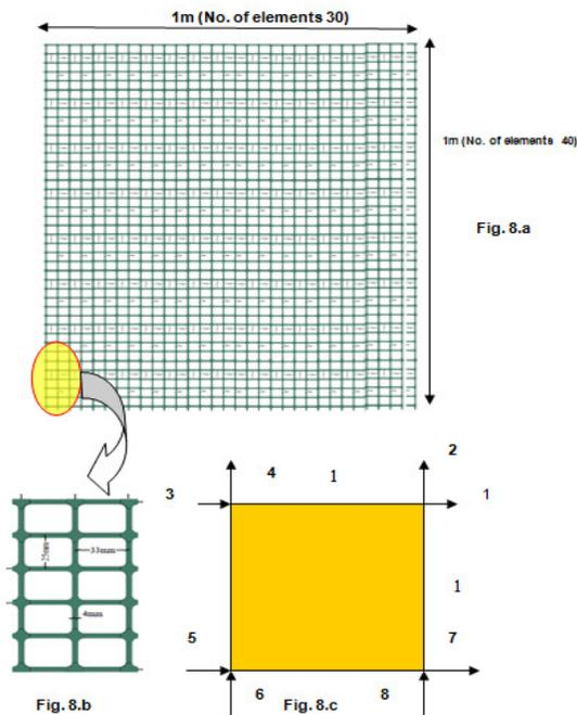
**Fig. 8.** Details of Geogrid and Macro element (a) Geogrid of size 1m x 1m with apertures (b) Geometrical details of geogrid (c) Geogrid represented as macro element of size 1m x 1m.
