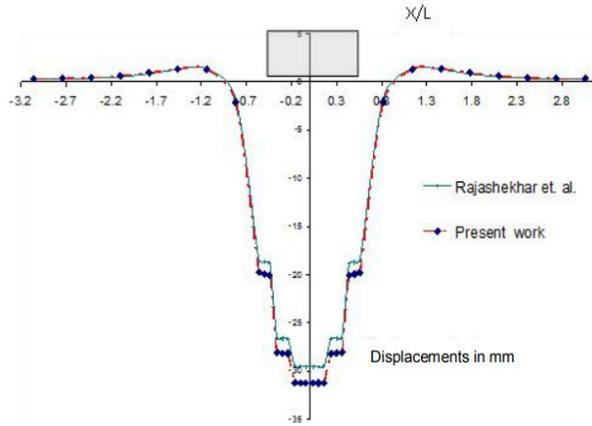
**Fig. 5.** Comparative settlements in mm at the centre in the present work and the referred work (Swamy *et al.* (2011)).
