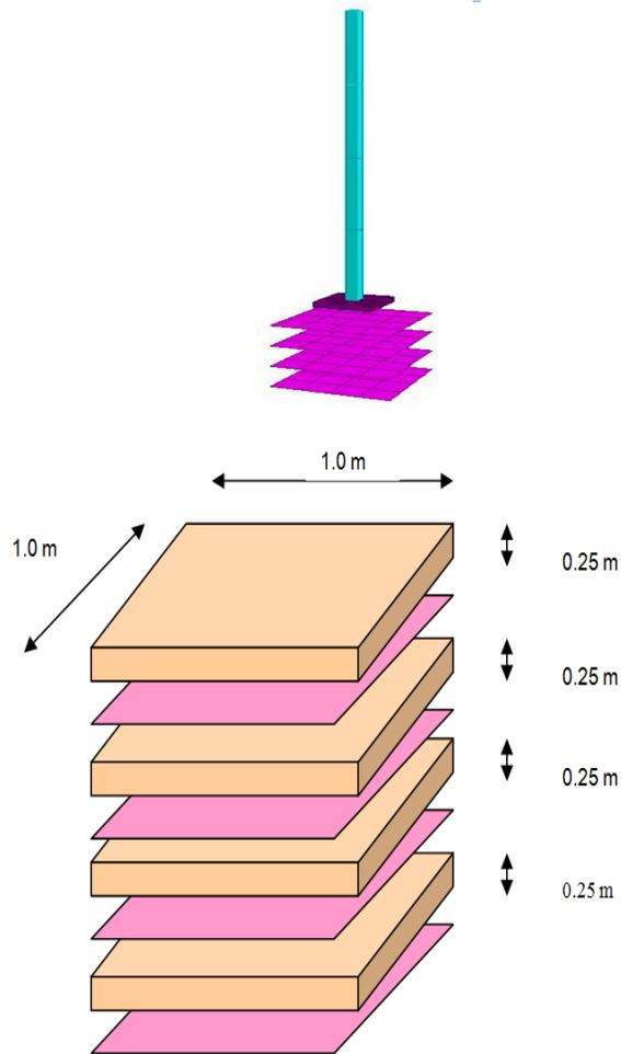
**Fig. 7.** Arrangement of geogrid (a) Modelling of column-foundation- Geogrid (b) soil-geogrid arrangement represented as macroelement in RSSI analysis.
