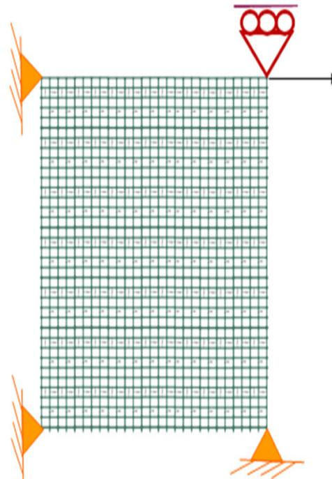
**Fig. 10.** Evaluation of first column elements of stiffness matrix of macro-element.
