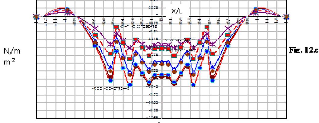
Fig. 12. Vertical stresses in  $\text{N/mm}^2$  linear RSSI analysis (a) Contours of vertical stresses at footing level (b) Vertical stresses along longitudinal section at centre (c) Vertical stresses at foundation level along longitudinal sections for different values of  $Z/L$ .
